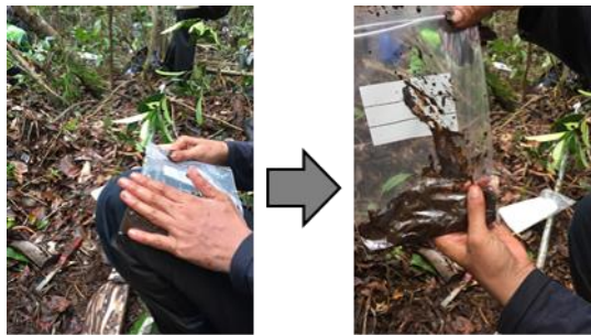
Air is removed from a soil sampling bag.
