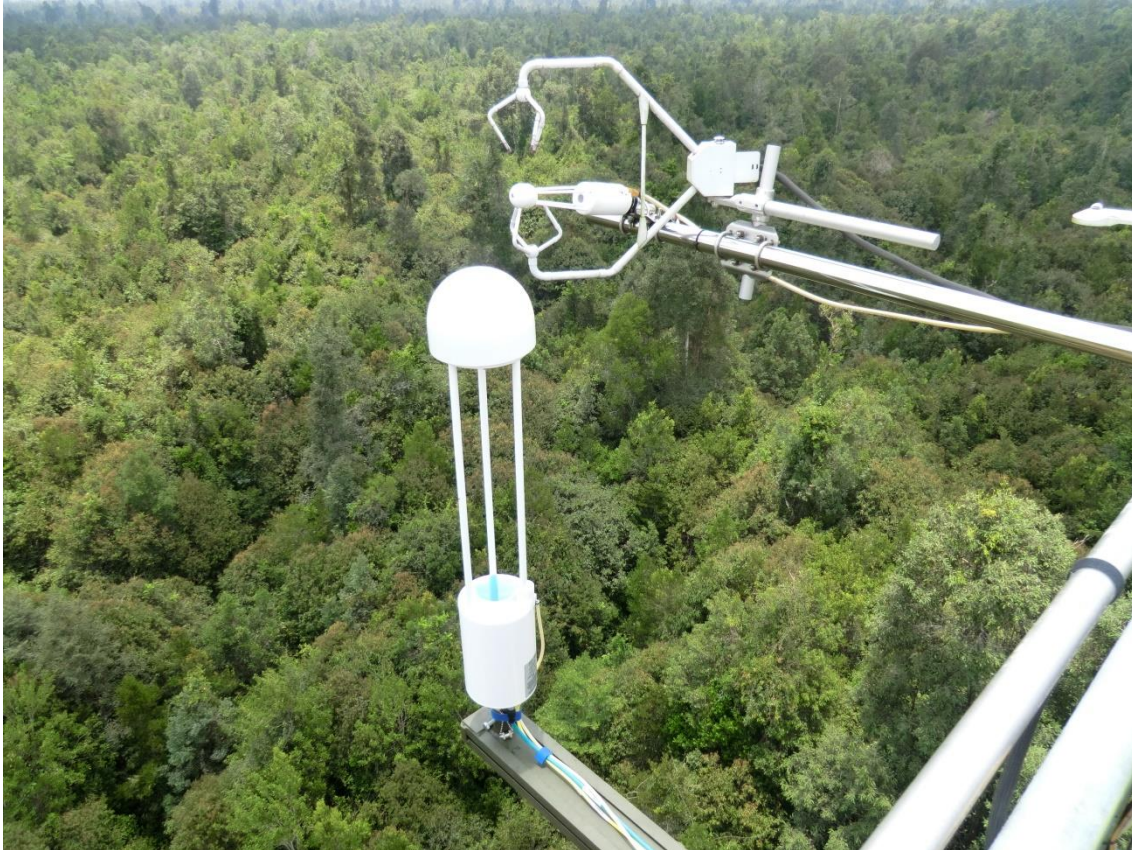
Figure 4.4: An eddy covariance system installed above a peat swamp forest. The front white system is an open-path \text{CH}_4 analyzer (LI7700)
