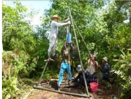
Figure 3. Works of the standard penetration test (SPT)
