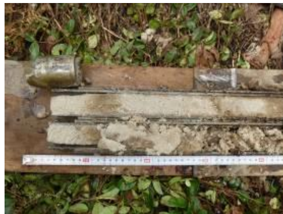
Figure 7. Sand collected by SPT sampler
