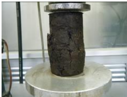
Figure 4. Specimen after unconfined compressive strength test
