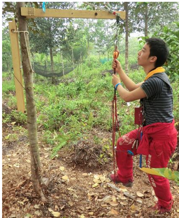
Figure 3. The tree bending test on a trunk of Shorea balangeran
