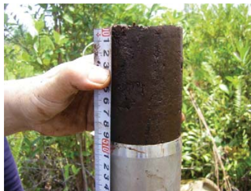
Photo1. Peat sample being pushed out of the sampling tube (GL-1.13m to 1.22m)
